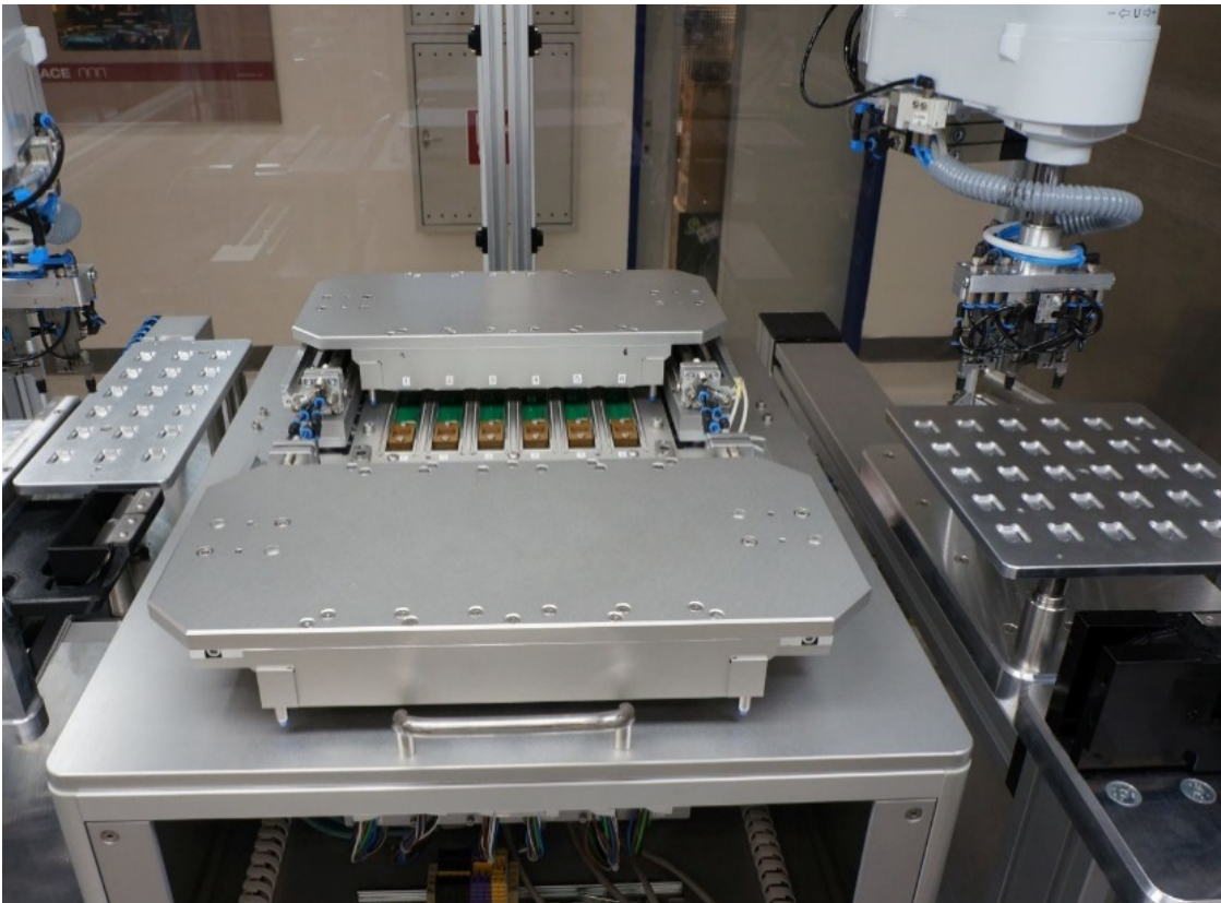
Figure 26: Automatic test equipment for module test
