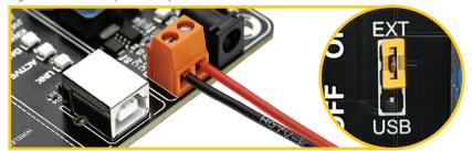
Figure 4: Powered by laboratory PSU
