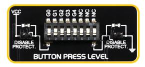
Figure 17: Button press level DIP switch
