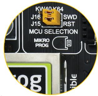
Figure 12: Target MCU selection jumpers
