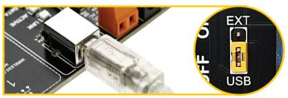
Figure 2: Powered by USB
