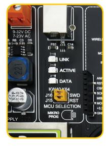
Figure 10: Programmer LEDs
