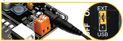
Figure 3: Powered by wall-adapter
