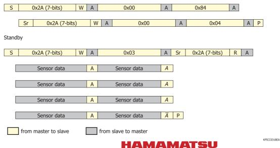
Condition 2: [Fixed time mode, Tint=01 (1.0 ms), integration time=1.0 ms/ch]
