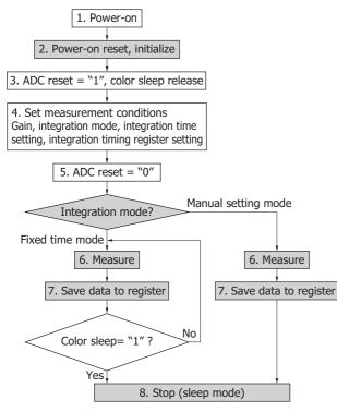
After power-on, the built-in power-on reset circuit operates to set all registers to their initial conditions (2.).
