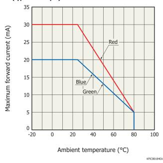
LED power dissipation vs. ambient temperature (typical example)
