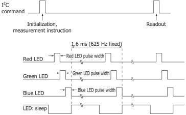
The 3-color LED emits light in the order red, green, and blue. The light emission pulse width can be set in the range of 0  $\mu$ s to 240  $\mu$ s in 16- $\mu$ s steps (16 levels total). The light emission pulse width can be set for each color. The light emission cycle is fixed at approximately 1.6 ms, and the drive current is fixed at 8 mA.
