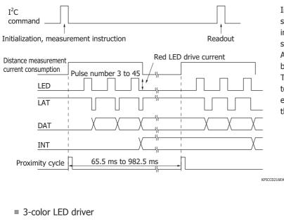
In the proximity sensor, the light emission pulse count is designed to be adjustable in integer multiples of 3 from 3 to 45 in order to increase measurement precision. The interrupt signal (INT) is set to 1 only when all pulses are detected.
