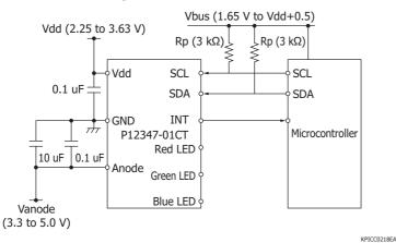
Note: When the LED is emitting light or when the proximity sensor is in use, do not externally drive the LED. Set the LED's anode voltage to 3.3 V or higher.
