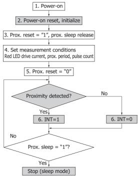
With the initial settings, the proximity sensor is in sleep mode. Therefore, first disable the sleep mode (3.). Next, set the drive current, pulse count, pulse cycle, and the like. Then, release the reset to start measuring (4. 5.). Proximity sensor continues to measure until it is set to sleep mode. To end measurement, enable sleep mode.
