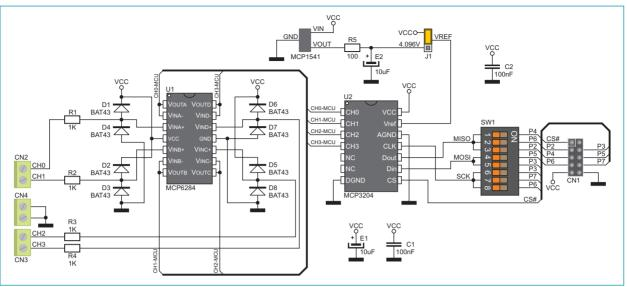
Figure 3: EasyADC additional board connection schematic
