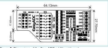
Figure 2: Dimensions of the EasyADC additional board
