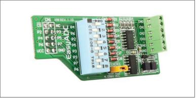
Figure 1: EasyADC additional board
