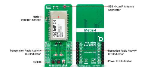
Communication between the Metis-I and the host MCU is made through a UART interface, using the standard UART RX and TX pins and hardware flow control pins (CTS/RTS). The module communicates at 115200bps by default, allowing efficient data exchange. The board also includes a reset (RST) pin for resetting the module. There are two LED indicators for user interaction: an orange TX LED signaling transmission activity and a yellow RX LED indicating reception.
