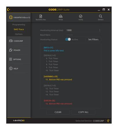
SWO [Serial Wire Output] trace is used to display various SWO-related messages in the Menu item section of the CODEGRIP Suite. The ARM SWO trace port uses a single pin to stream out data packets over 32 different ports, using the specified clock rate. The SWO is a part of the ARM<sup>®</sup> CoreSight Debug module which is incorporated in most of the MCUs based
