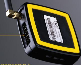
The CODEGRIP device is equipped with the target MCU connector, which contains JTAG/SWD and power supply pins. This connector is used to interface the CODEGRIP device with the target MCU, allowing it to perform programming and debugging operations, to provide the power supply for the target MCU, and to be used as the power input when the CODEGRIP device is powered from the connected development board.
