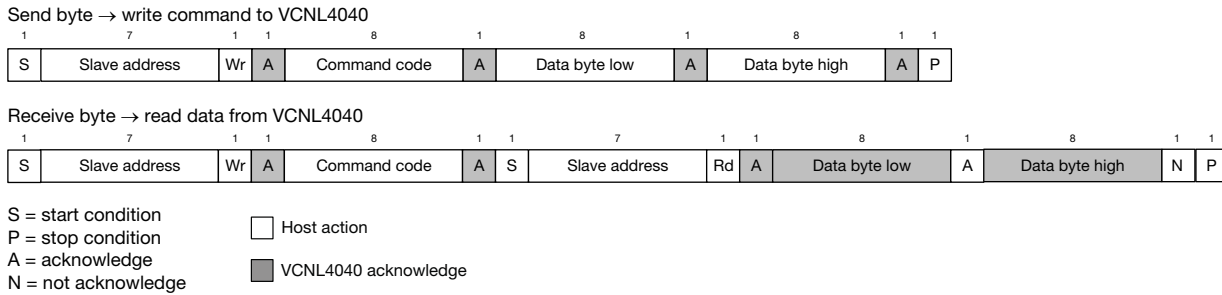
Fig. 12 - Write Word and Read Word Protocol
