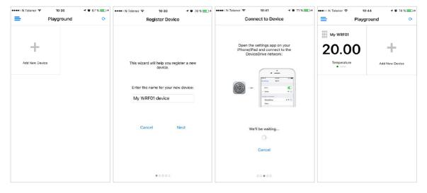
The device state is shown in the app after the introspect and current state have been sent to the cloud. The next section describes how to simulate device behavior.
