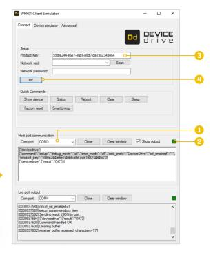
It is possible to mix up the host port and the log port in the two windows. It is recommended to plug in the HOST port first, and then select the port in the host communication window before connecting the log port.
