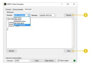
NOTE: This software strips your message of all <CR> <LF> characters before sending them to the WRF01. In a real-world application, do not use these characters in a WRF01 command. They have to comply exactly with the serial specification. If a command does not start with exactly {"devicedrive": the message will be interpreted as a cloud message transfer, and not a WRF01 command.
