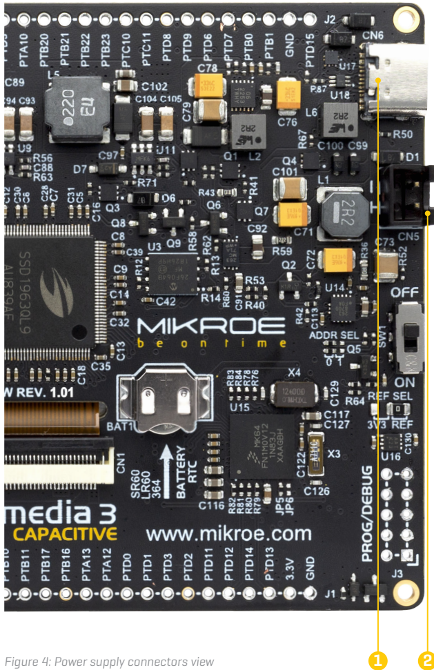
Figure 4: Power supply connectors view
