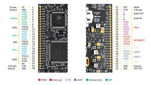
Figure 14: 1x26 pin header view
