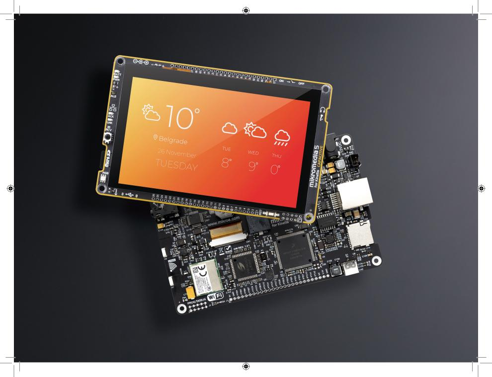
mikromedia 5 for Kinetis CAPACITIVE is a compact development board designed as a complete solution for the rapid development of multimedia and GUI-centric applications. By featuring a 5" capacitive touch screen driven by the powerful graphics controller that can display the 24-bit color palette (16.7 million colors), along with a DSP-powered embedded sound CODEC IC, represents a perfect solution for any type of multimedia application.
