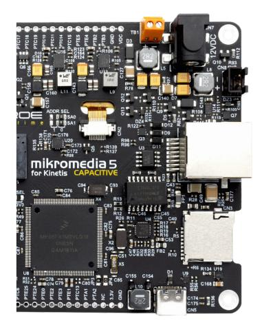
Figure 3: Power supply unit view
