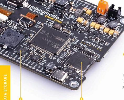
Figure 9: MicroSD card slot view
