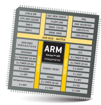
Figure 1: STM32F407ZGT6 MCU block schematic
