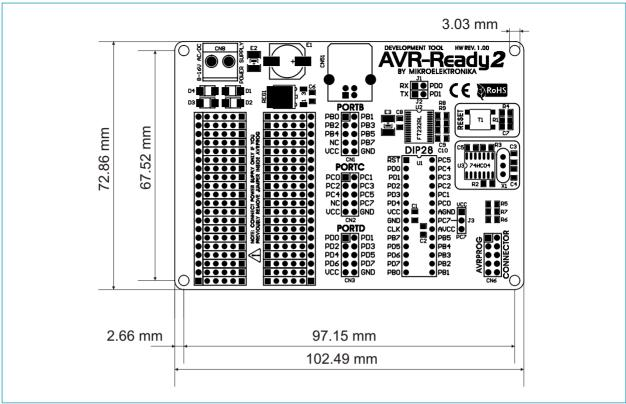
Figure 5: Additional board dimensions
