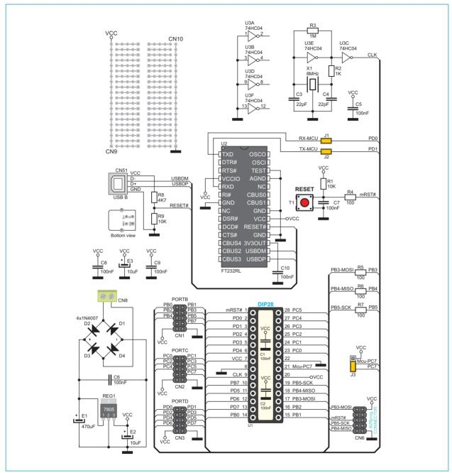
Figure 4: Additional board connection schematics
