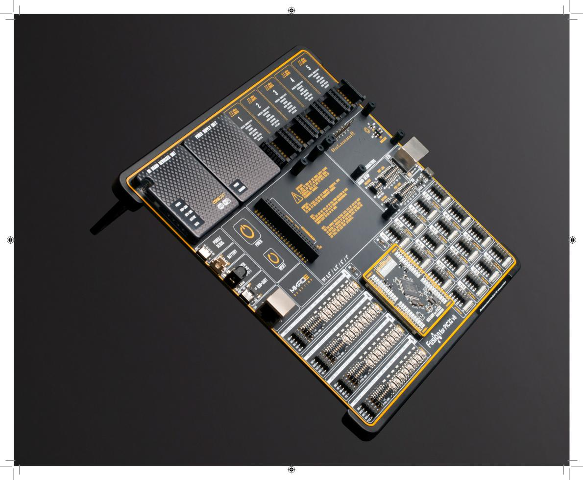
Fusion for PIC32 v8 is a development board designed for rapid development of embedded applications. Redesigned from the ground up, it offers broad set of standard, as well as several unique features never seen before in the world of embedded electronics: programming and debugging over WiFi network, support for a large number of Microchip's PIC32 microcontrollers regardless of their pin number and more.
