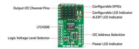
I2C MUX 5 Click communicates with MCU using the standard I2C 2-Wire interface with a frequency up to 400kHz. It also has three address pins (A0, A1, and A2 that provides 27 specific addresses) programmed by the user to determine the value of the last three LSBs of the slave address selected by onboard SMD jumpers labeled as ADDR SEL, allowing selection of the slave address LSBs.
