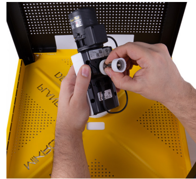
Figure 7: Screw the camera to the mounting bracket
