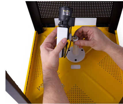
Figure 8: Screw the camera to the camera holder
