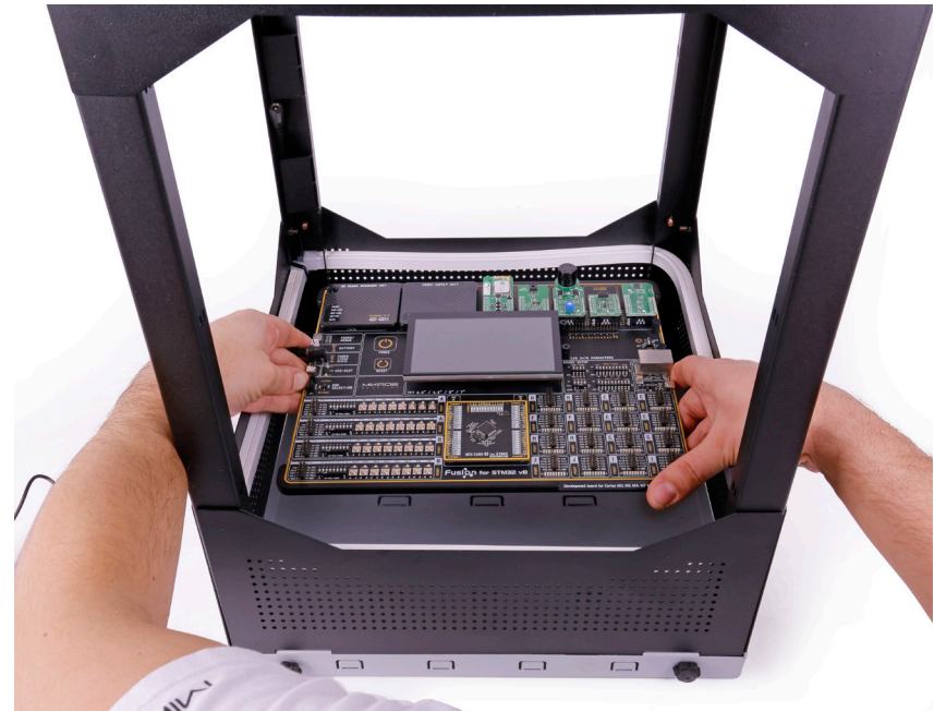
Figure 5: Placing development board into the metal base
