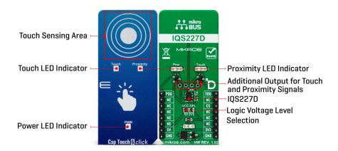
Touch and proximity features, alongside its mikroBUS<sup>™</sup> pins, marked TOU and POU, only used to communicate with MCU, also have their corresponding LED indicators, labeled Touch and Proximity, reporting the activity of these features. If a touch/proximity event is detected on the onboard sensing pad, the state of the corresponding LED will be changed, indicating an activated channel.
