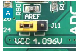
Figure 7-4: The position of jumper J11
