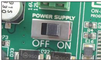
Figure 1-3: Power supply on/off switch
