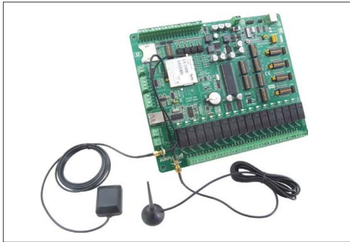
Figure 9-6: Telit's module with connected antennas
