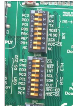
Figure 8-2: DIP switches SW9 and SW10
