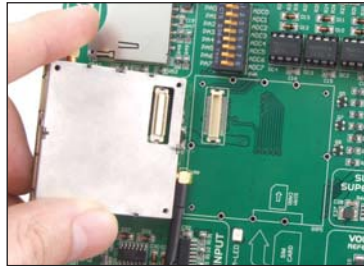
Figure 9-2: Connecting Telit's GM862 module
