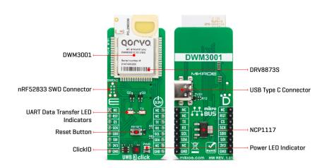
The DWM3001 UWB transceiver also incorporates the LIS12DH, a low-power three-axis linear accelerometer from STMicroelectronics. It is necessary as RTLS tags commonly use accelerometers to initiate UWB ranging only when a tag moves so that battery life can be extended by staying in the lowest power mode by default. Near-field communication type 2 (NFC-A) can be used by adding an NFC antenna to the TP1 and TP2 pads.
