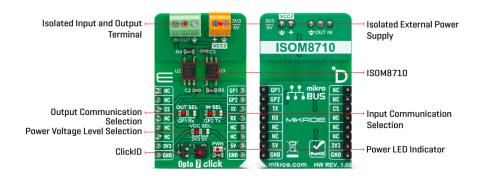
Opto 7 Click can use general-purpose IO to communicate with the host MCU over the GP1 and GP2 pins. It can also be used for a standard UART communication isolation with commonly used UART RX and TX pins. The selection can be made over the OUT SEL and IN SEL jumpers. Both should be in a proper position for the communication to work.
