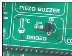
Figure 6-2: Temperature sensor DS1820 is connected
