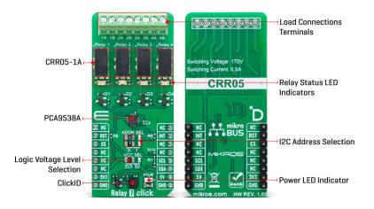
The CRR05-1As also feature a high insulation resistance of a typical  $1013\Omega$ . Its electrical specifications include a coil voltage of 5VDC, a coil resistance of  $150\Omega$ , a single-pole singlethrow normally open (SPST-NO, 1 Form A) contact form, and maximum rated power of 10W/170VDC/0.5A.
