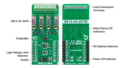
The 9913-05-20TRs also feature a high insulation resistance of a minimum of  $1011\Omega$  and an external magnetic shield. Its electrical specifications include a coil voltage of 5VDC, a coil resistance of  $200\Omega$ , a single-pole single-throw normally open (SPST-NO, 1 Form A) contact form, with the contact current rating capped at 250mA and the switching voltage limited to 100VAC and 100VDC.
