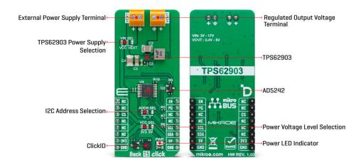
Communication with the Buck 15 Click is conducted through a standard 2-wire interface linked to the <u>AD5242</u>, allowing the host MCU to adjust the output voltage. The device's I2C address is configurable via the ADDR SEL jumper, with a default setting of 0. This Click board™ also features a power-good (PG) pin that indicates when the output voltage falls outside the predetermined window threshold and an EN pin, which serves as a precision regulator-enable input.
