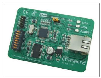
Figure 1: Serial Ethernet2 additional board
