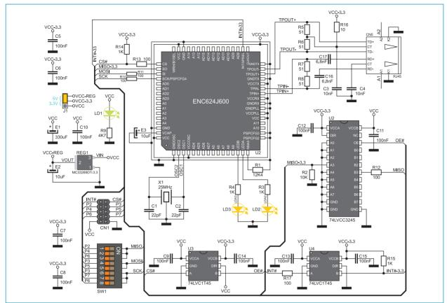
Figure 3: Serial Ethernet2 board connection schematic
