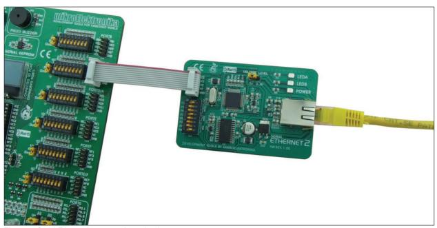
Figure 4: Serial Ethernet2 connected to a development system
