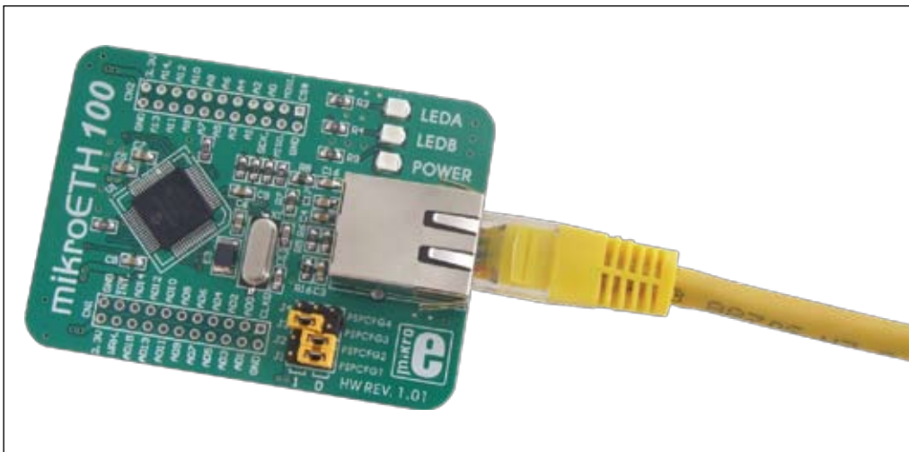
Figure 4: mikroETH 100 connected to the Ethernet cable
