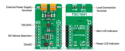
Current 12 Click uses a standard 2-wire I2C communication protocol to enable the host MCU to control the TSC1641. The I2C interface supports clock frequencies of up to 1MHz, with the I2C address selectable via the ADDR SEL jumpers. The alert interrupt ALR pin allows the assertion of several alerts regarding voltage, current, power, and temperature, with thresholds that can be set for each parameter in a specific register.
