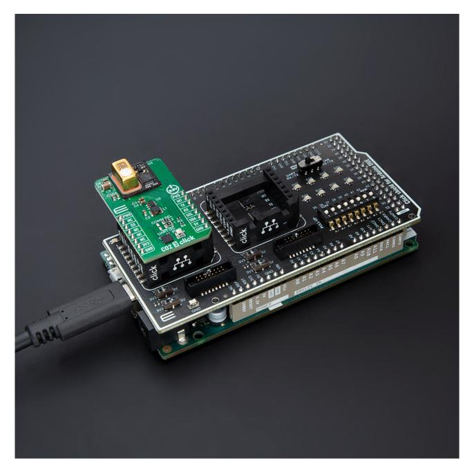
When the USB type C is connected to the Click Shield, the PWR diode will glow Blue, and at this setup, the connected Arduino DUE baseboard and all mikroBUS $^{\text{m}}$  sockets will be powered from it.
