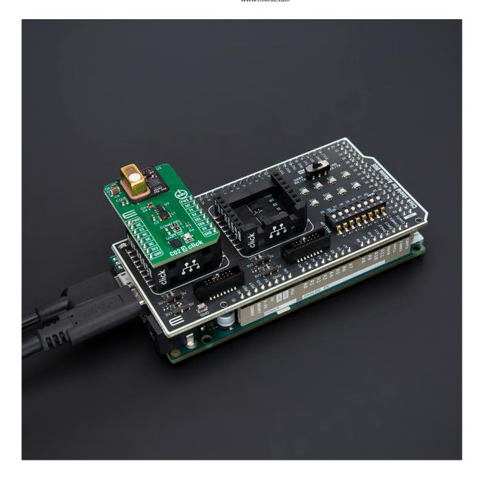
When the USB type C is connected to the Click Shield and the other USB is connected to the Arduino DUE board, the PWR diode will glow Cyan, and at this setup, the mikroBUS $^{\text{m}}$  sockets are powered from the Click Shield.
