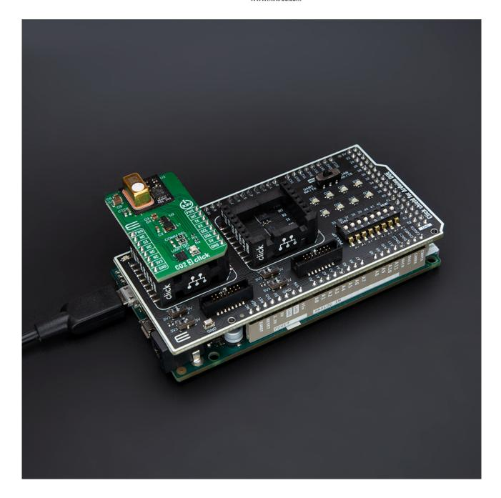
When the USB is connected to the Arduino DUE board, the PWR diode will glow Green, and at this setup, the Arduino DUE baseboard itself will be supplied, and it will provide power to the Click Shield, including all mikroBUS™ sockets.
