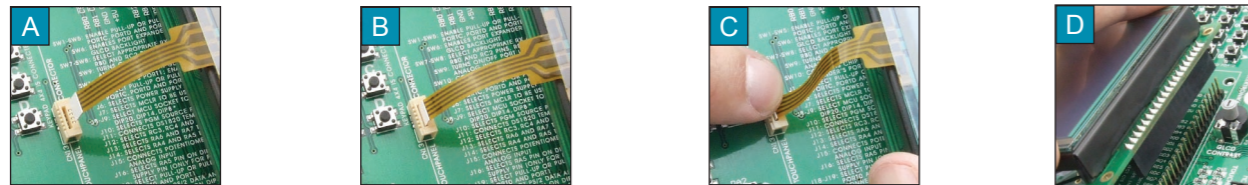
Figure 16-3: Connecting touch panel
