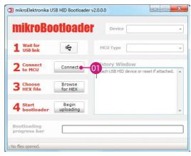
Figure 1-1: USB HID mikroBootloader window
