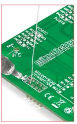
Figure 3-4: soldering 2x5 male header on the pads
