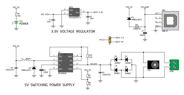
Figure 1-4: Power supply schematic
