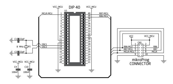
Figure 3-6: mikroProg<sup>™</sup> programmer connection schematic
