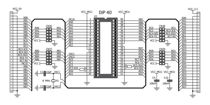
Figure 6-1: Schematic of pin headers and connection pads
