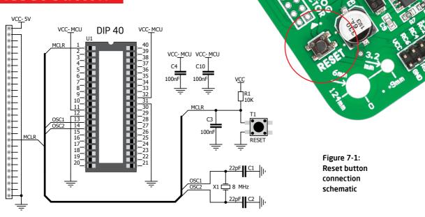
Ready for PIC\* board has a specialized reset circuit with a high-quality reset button which can be used to reset the program execution of the microcontroller. If you want to reset the circuit, press the on-board RESET button. It will generate a low voltage level on the microcontroller reset pin (input). In addition, a reset can be externally generated through **MCLR pin** on 1x28 connection pads.
