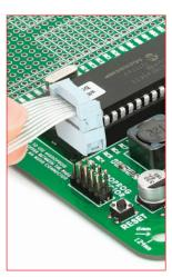
Figure 3-5: Connecting mikroProg™ programmer
