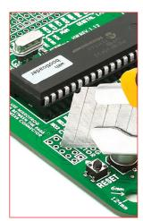
Figure 3-2: cutting copper between pads
