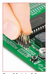
Figure 3-3: placing 2x5 male header
