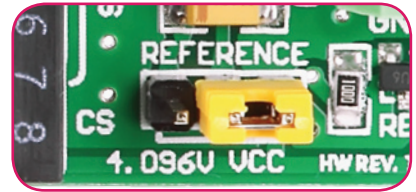
Figure 4-2: Ref. voltage is VCC
