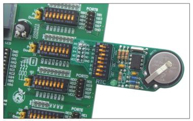
Figure 4: RTC board connected to a development system
