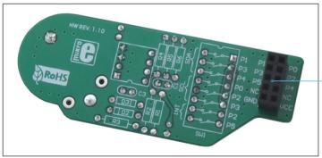
2x5 female connector enables the additional board to be connected to a development system
