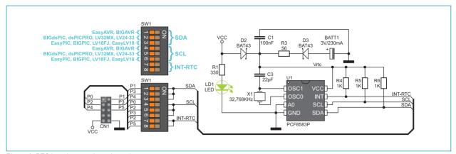
Figure 3: RTC board connection schematic
