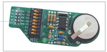
Figure 1: RTC board
