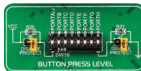
Figure 6-5: Button press level DIP switch (tri-state)
