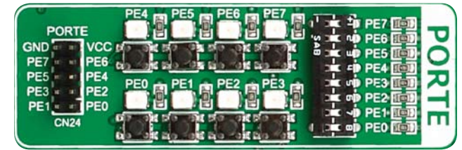
Figure 6-1: I/O group contains PORT header, tri-state pull up/down DIP switch, buttons and LEDs all in one place
