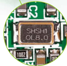
Figure 5-1: 8MHz crystal oscillator
