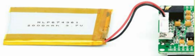
Figure 1-2: Connecting Li-Polymer battery
