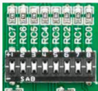
Figure 6-2: Tri-state DIP switch on PORTC
