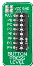
Figure 6-5: Button press level DIP switches (tri-state)
