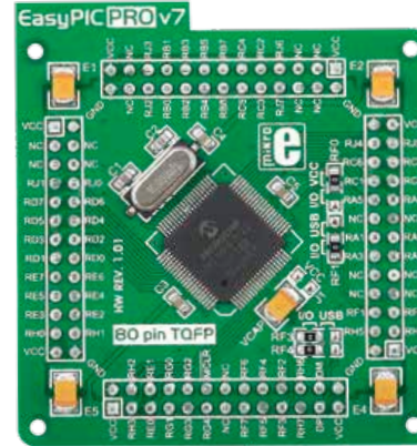
3 Figure 4-7: Standard 80-pin MCU card with PIC18F8722 .
