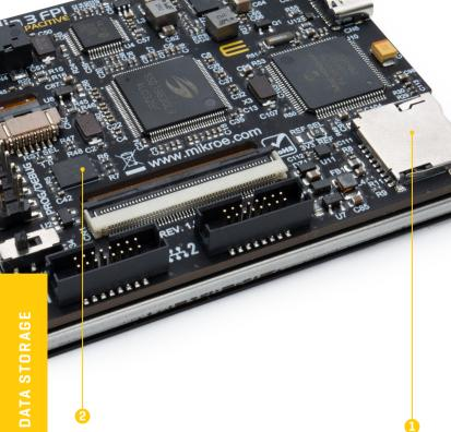
Figure 10: MicroSD card slot view
