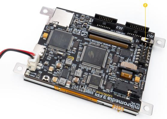
Figure 8: Battery power supply connection
