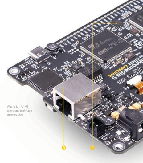
It allows mikromedia 5 to connect to an Ethernet network over the standard RJ-45 connector **(3)**. Ethernet lines are further protected from electrostatic discharge (ESD) by a pack of TVS diodes. mikromedia 5 is equipped with two LED indicators, which are located on the front side. They are used to signal status and data traffic.
