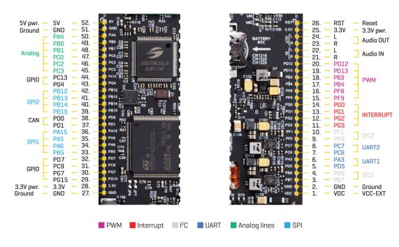
Figure 14: 1x26 pin header view
