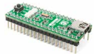
MIKROE-1367 MINI-M4 for STM32 contains STM32F415RG (ARM ® Cortex ™ -M4)
