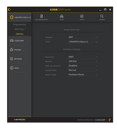
To use the SWO Tracing, the programming protocol must be set to SWD. Not all ARM® MCUs support the SWO Trace. For more information about the SWO Trace capabilities, please consult the datasheet or the reference manual of the used MCU.
