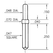
**Description:** 0600 - Solder Mount PCB Pin **Packaging:** Packaged in Bulk
