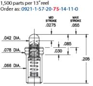
Solder mount in .070 min. mounting hole
