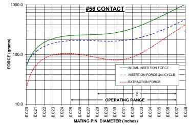
The insertion/extraction/normal force characteristics above were derived using 30 microinch gold plated contact and polished steel gauge pins having a bullet-shaped tip.
