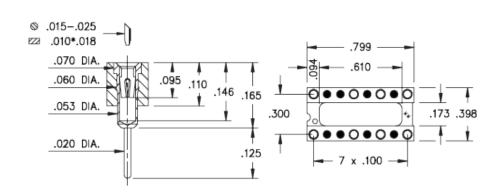
**Description:** DIP Dual In Line Socket Selectively Loaded Socket for Dual In Line Relays Open Frame Through Hole Plating Code: 13 Shell Plating:  $10~\mu$ " Gold over  $100~\mu$ " Nickel
