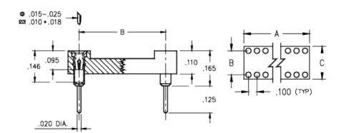
DIP Dual In Line Socket
