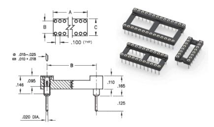
**Description:** DIP Dual In Line Socket Standard Solder Tail Open Frame Through Hole Plating Code: Shell Plating: 200 µ" Tin (matte finish) over 100
