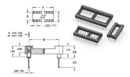
DIP Dual In Line Socket Standard Solder Tail Open Frame Through Hole Plating Code: Shell Plating: 200 μ" Tin/Lead(93/7) over 100 μ" Nickel Inner Contact Plating: 30 μ" Gold over 50 μ" Nickel Packaging:
