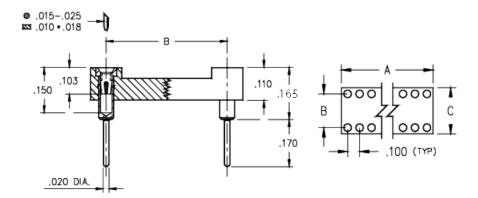
**Description:** DIP Dual In Line Socket Long Solder Tail DIP Open Frame Through Hole Plating Code:
