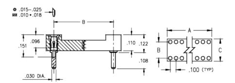
**Description:** DIP Dual In Line Socket Low Profile Solder Tail DIP Open Frame Through Hole Plating Code:
