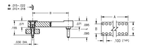
DIP Dual In Line Socket
