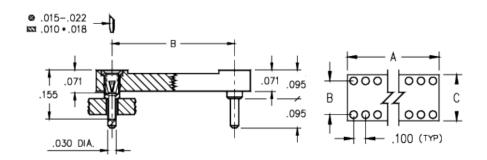
DIP Dual In Line Socket
